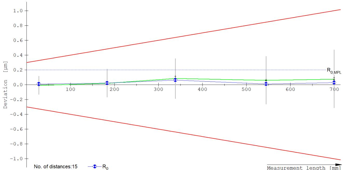
The bar lengths represent the uncertainty intervals  $+/- U(E)$ , and the central points represent the values obtained for the errors of indication.
