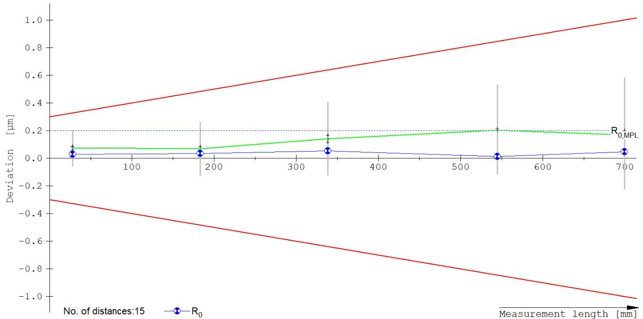
The bar lengths represent the uncertainty intervals  $\pm U(E)$ , and the central points represent the values obtained for the errors of indication.
